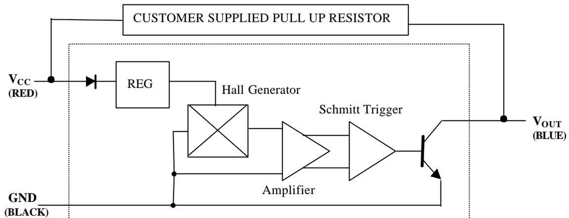
NOTE: A pull-up resistor is required on the open collector output to establish a quiescent voltage level. The pull-up resistor also provides faster rise times and improves noise immunity. Contact the factory for application assistance.
